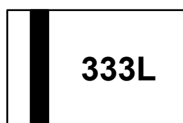
333L= Device Marking Code Bar denotes Cathode
